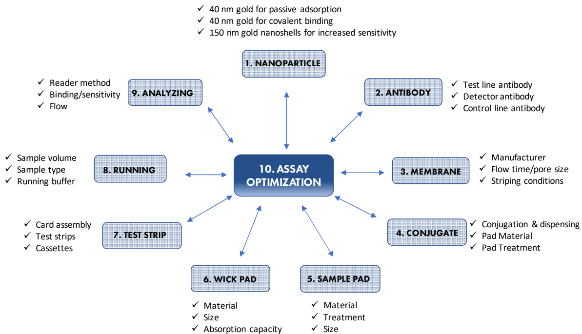
Figure 16: Iterative optimizations that are performed to maximize performance of lateral flow assay. The steps outlined in this handbook are often revisited multiple times throughout the development cycle until the assay results meet your desired requirements.
