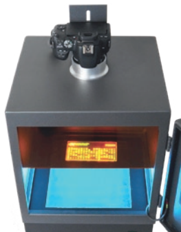
Use the additional amber shield to cut out DNA bands
