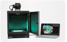
The FAS-Digi PRO is composed of a huge transilluminator with an illuminated area of 26 x 21 cm. The dark hood can be easily removed, which allows a very easy excision of DNA bands.
