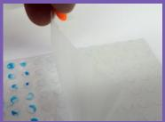
• Remove protective film from both the Film Base and the Cover Film (indicated by round red stickers).
