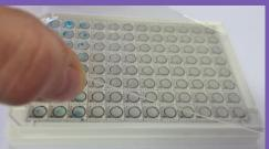
• Cover the Film Sandwich with the Evaporation Cover (Plain - not printed).
