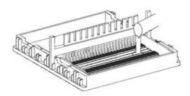
Make sure there are no air bubbles after pouring, especially around the comb. Remove them with a pipette tip, while the agarose gel is still liquid.
