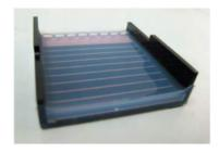
• Put the gel with the black gel tray in to the electrophoresis tank and apply samples and marker.
