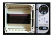
• Put the Illuminator lid on top of the electrophoresis tank. Make sure that the safety bars fit correctly into the slits of the power supply.
