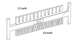
Place the comb into the casting stand. Place it in positions with the round marks of the stand to obtain equal intervals.
